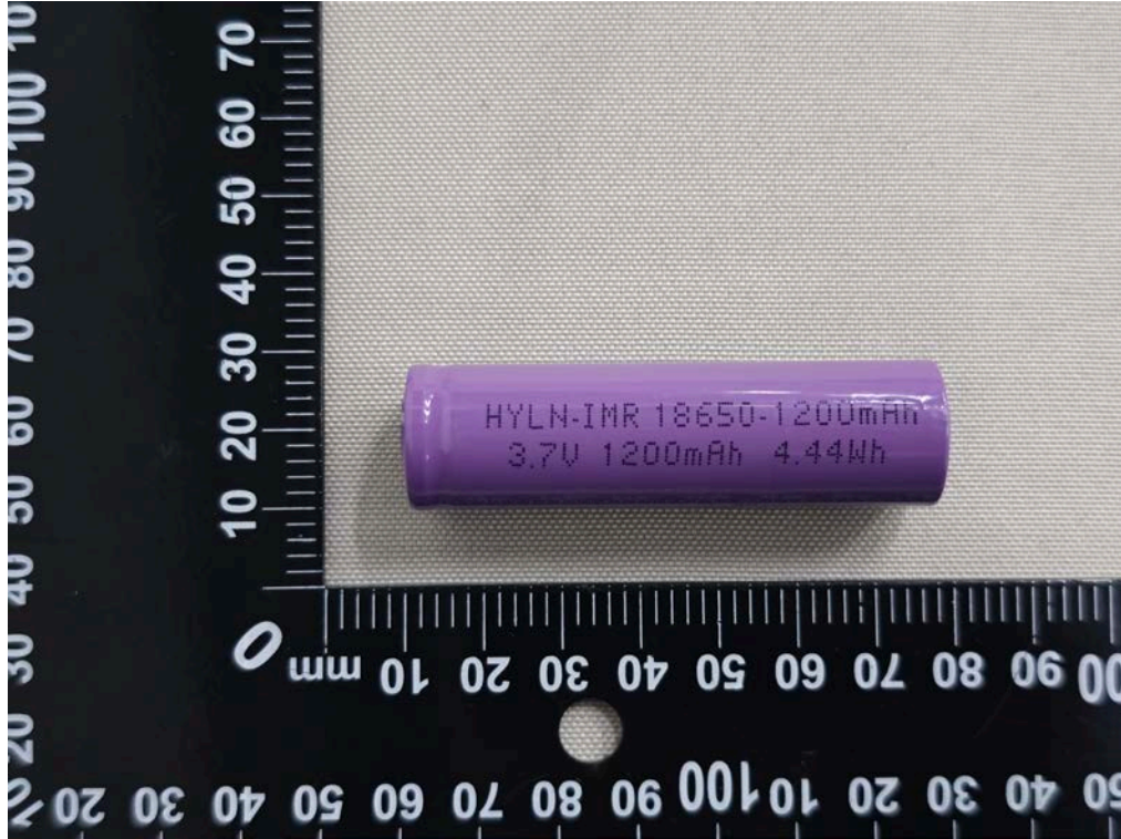
Figure 7 Front view of cell (Model: IMR18650-1200mAh)
