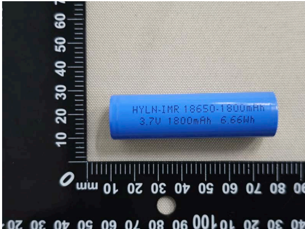
Figure 3 Front view of cell (Model: IMR18650-1800mAh)
