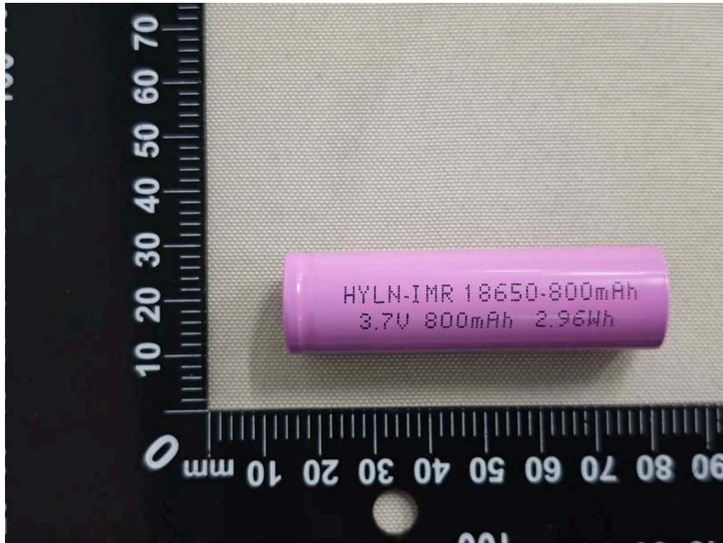
Figure 9 Front view of cell (Model: IMR18650-800mAh)
