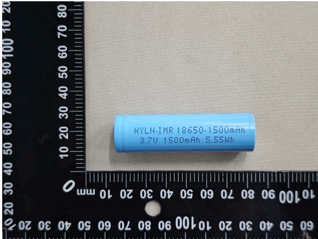
Figure 5 Front view of cell (Model: IMR18650-1500mAh)
